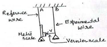
The experimental wire (B) is of uniform area of cross-section also carries a pan in which known weights can be placed. The vernier scale is attached to a pointer at the bottom of experimental wire B and main scale is fixed to the reference wire A.
